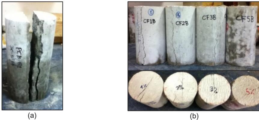
Figure 7. Broken samples following STS tests: (a) plain concrete (b) CFRC.
